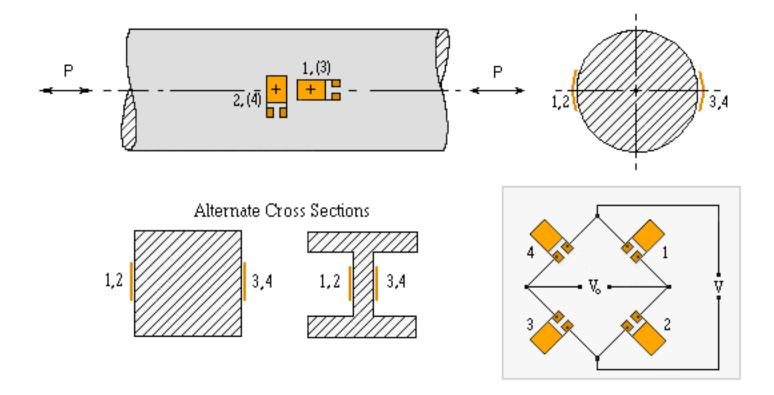
*Tension/Compression (Direct-Stress) Force Transducer*
