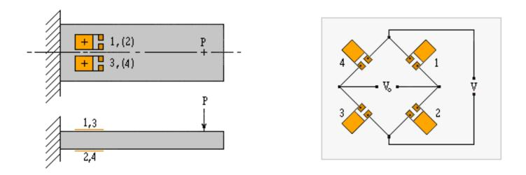
Cantilever Beam Force Transducer, with Full-Bridge Circuit for Doubled Output Signal (Dimensions same as <u>previous figure</u>)
