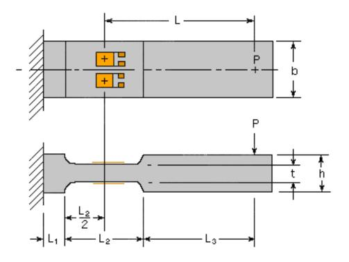
Mechanical Design of Cantilever Spring Element for Reduced Compliance. Deflection Under Load is a Function of b, t, h,  $L_1$ ,  $L_2$ ,  $L_3$
