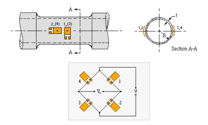
Pressure Transducer, Using A Thinned Pipe Wall.
