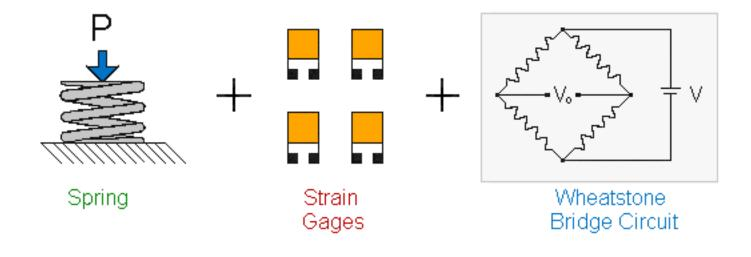
Principal Components of a Strain-Gage-Based Transducer
