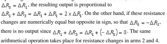
In contrast, resistance changes in adjacent bridge arms are subtracted algebraically. Therefore, if  $\Delta R_2 = \Delta R_1$  (in magnitude and sign), the bridge
