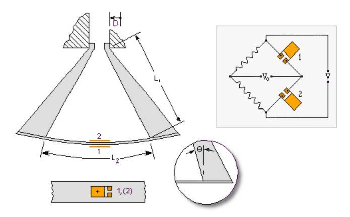
Principle Of Clip Gage For Displacement Measurement
