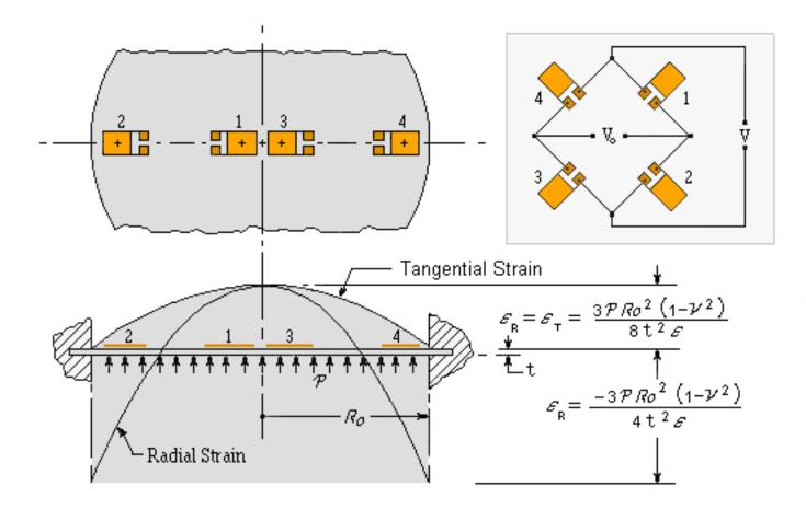
Diaphragm Pressure Transducer, With Strain Distribution And Gage Positioning
