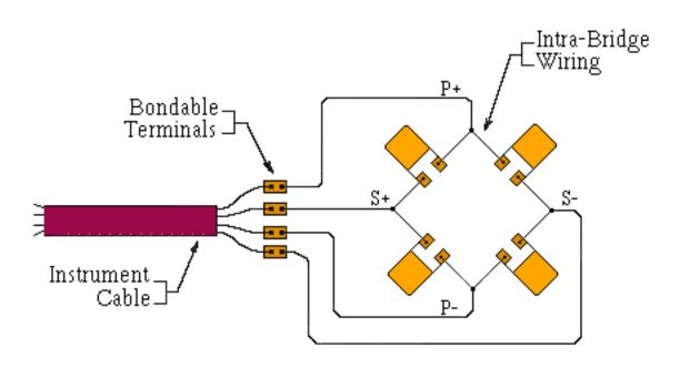
Typical Transducer Wiring Arrangement
